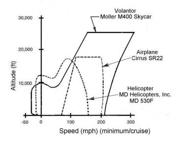
horsepower output per pound of engine weight together with a low engine cost per in horsepower. The figure below documents that there are no magical short cuts to generating viable VTOL aircraft. If one wants to operate at a Skycar® aircraft's speed and payload then the type of aircraft to achieve that goal is identified (ducted fan) as is
